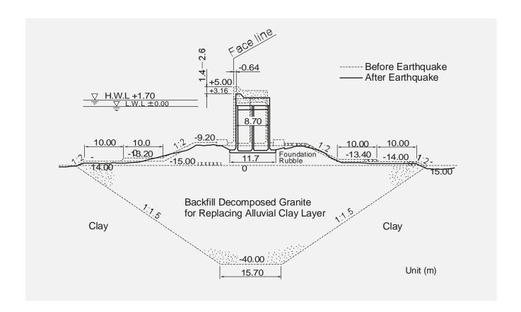
The analysis results in settlement of breakwater, associated with lateral spreading of rubble mound.
